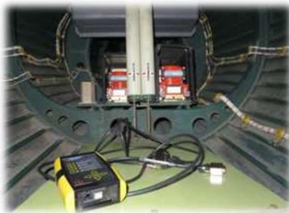
The AIC will download the data from the recorders “on-wing”, meaning that the download is conducted with the recorders left in the aircraft and using the aircraft’s electrical power. This process is used by the AIC whenever possible to minimise aircraft down time if the recorders had to be taken to the AIC Laboratory.
