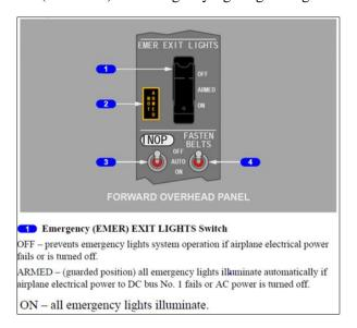
Figure 1: Cockpit Overhead Panel Emergency Light switch<sup>2</sup>
