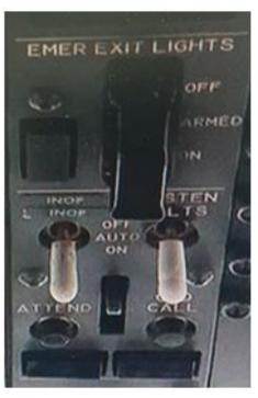
Figure 2: P2-PXE Cockpit Overhead Panel Emergency Light switch during the approach<sup>3</sup>
