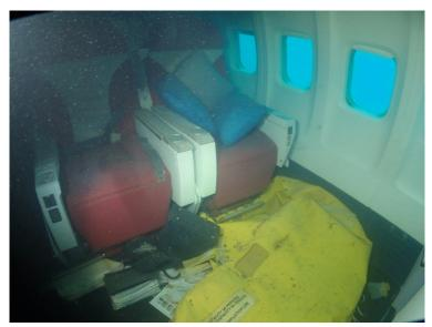
The investigation examined photographic evidence and found that two life rafts were in the water and one was on a seat in the over-wing exit row and had not been used because of the abundance of small rescue craft that came to the crash site. There was a 56-person life raft bag/cover laying on the floor in front of Business Class Seats 1A and 1B.
