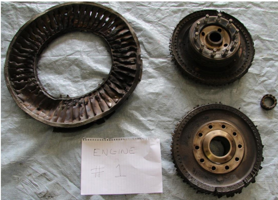
Figure 41: Left engine first and second stage power turbine and nozzle guide vanes
