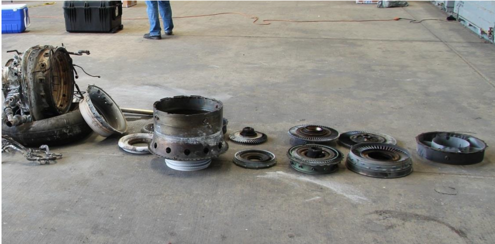
Figure 43: Disassembled right turbo-machinery section
