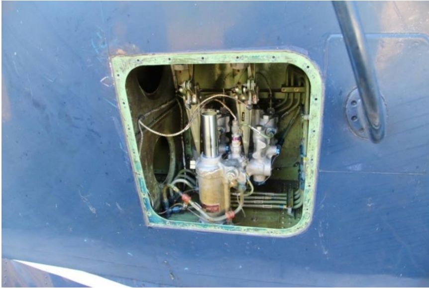
Figure 23: Missing panel on vertical stabiliser
