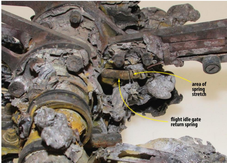
Figure 47: Close-up of power lever quadrant with flight idle return spring
