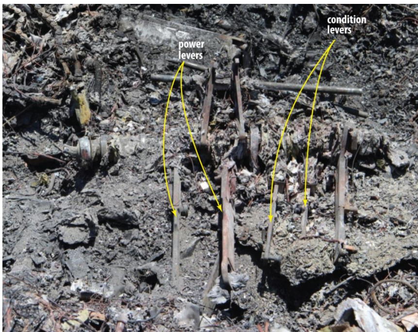
Figure 27: Power lever quadrant components as found on-site
