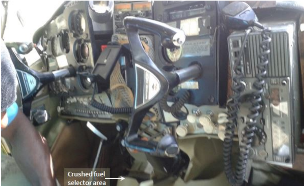
Figure 4. Damage to the cockpit area
