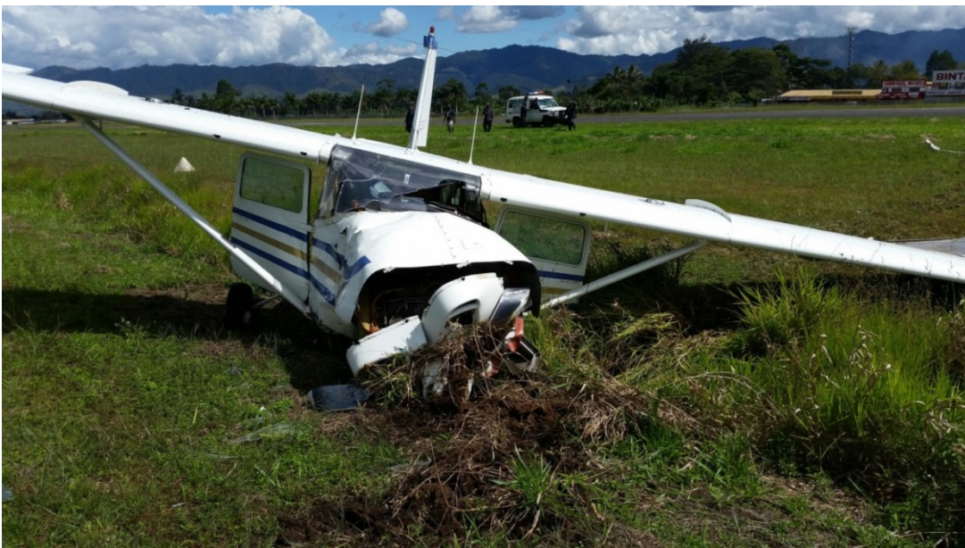
Figure 3: Damage to the propeller and the engine.
