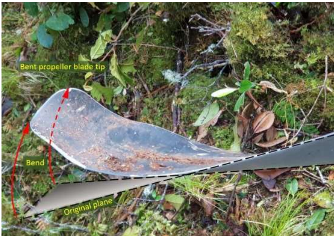
Figure 8: Propeller tip bending
