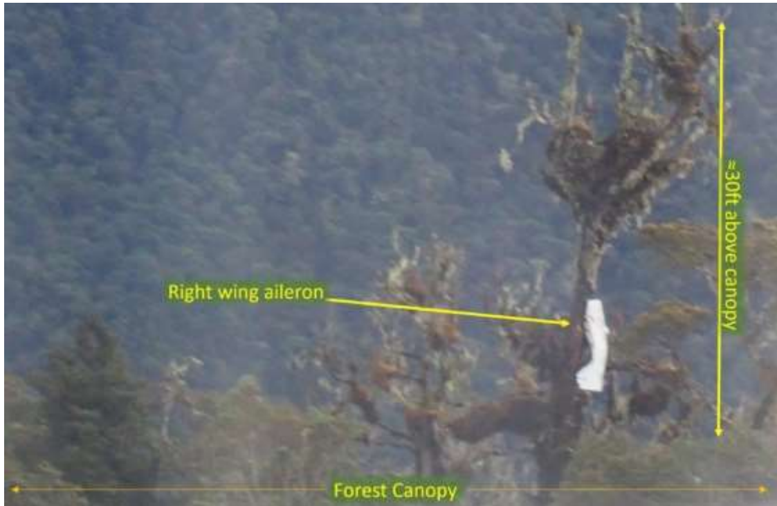
Figure 2: P2-ISM right aileron hanging from a tree.
