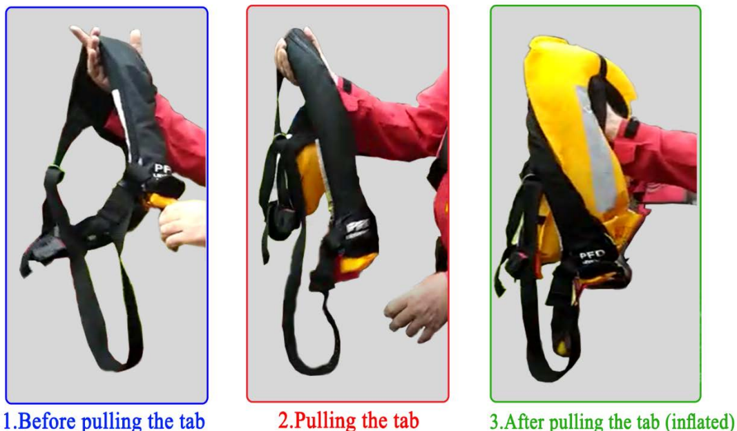
Figure 2: Testing the pilot's life jacket
