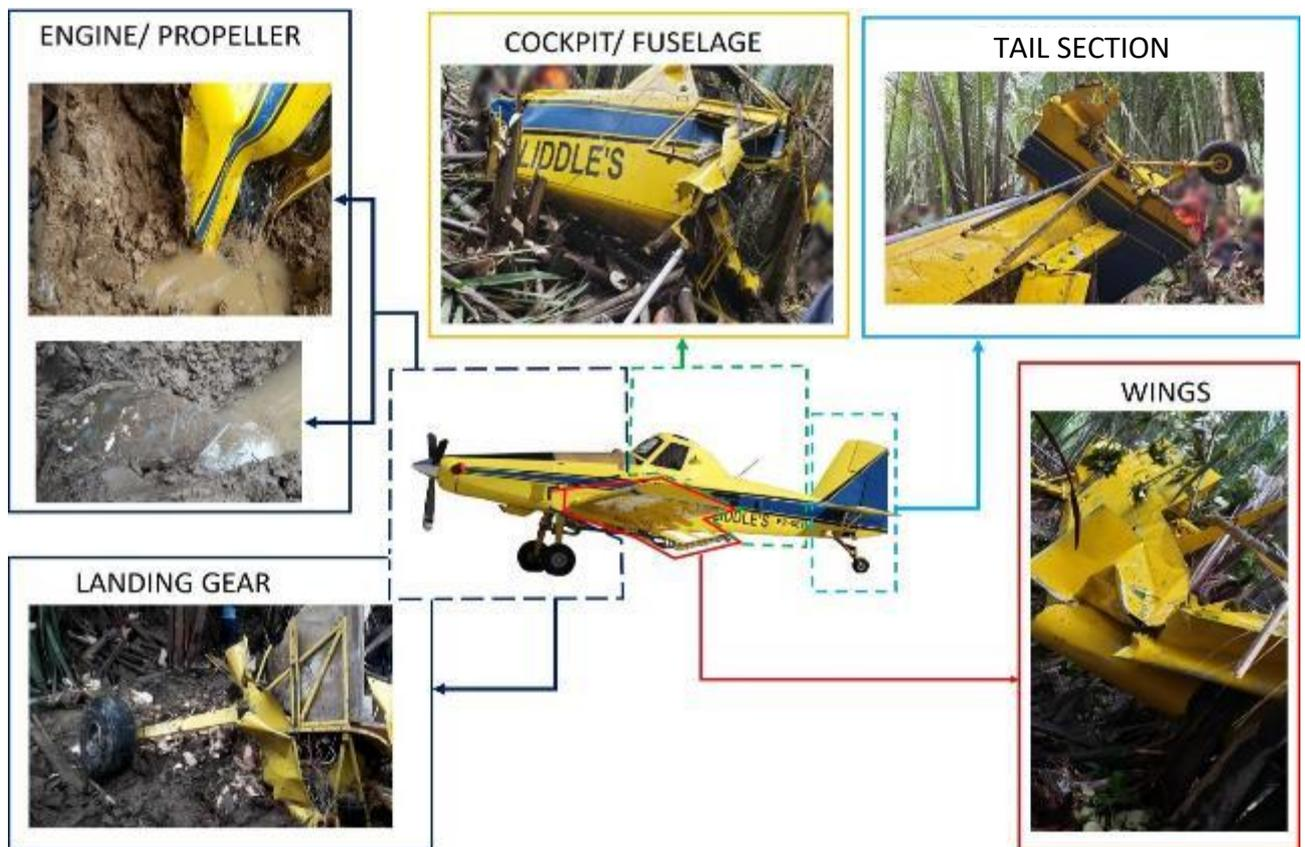
Figure 11: Wreckage distribution
