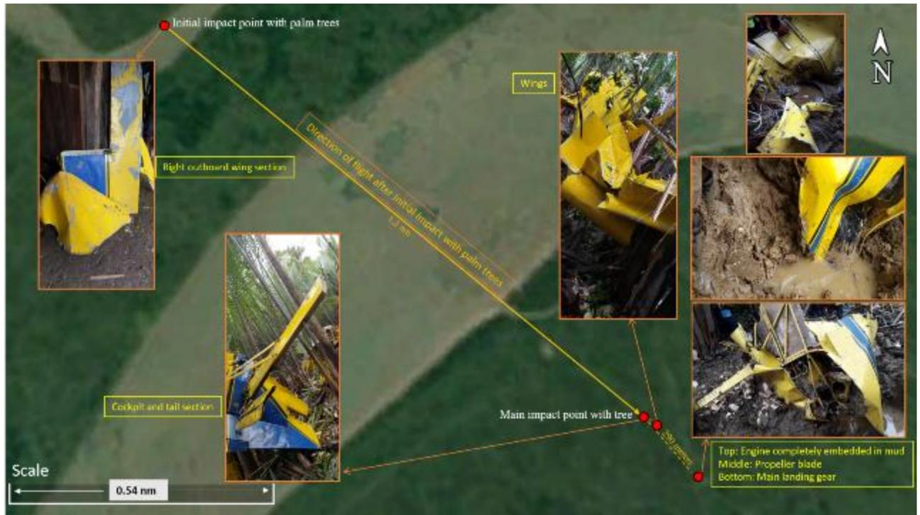
Figure 10: Depiction of wreckage trail along final flightpath
