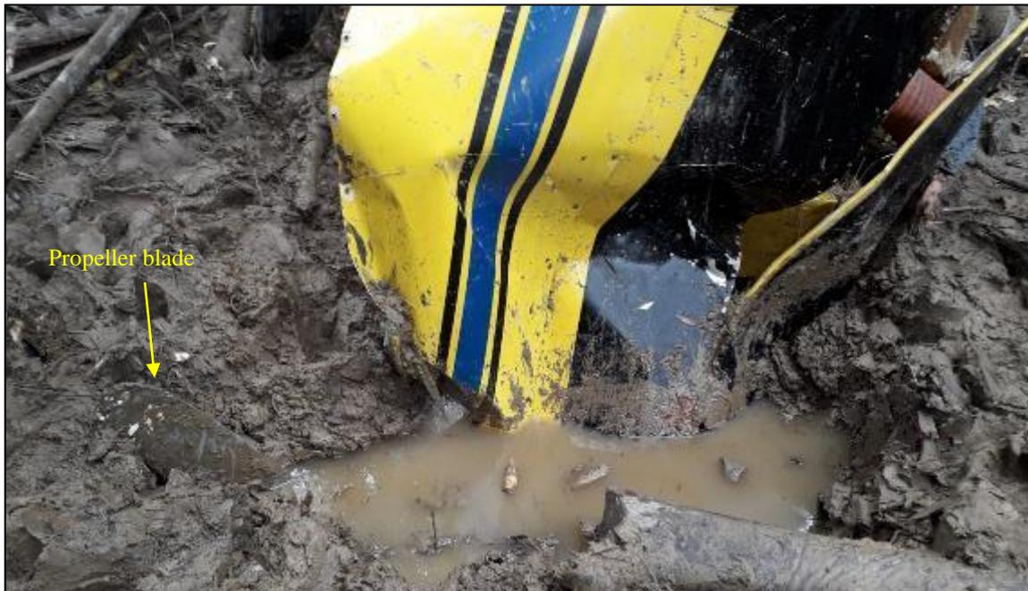
**Figure 15: Engine and propeller section embedded in mud**
