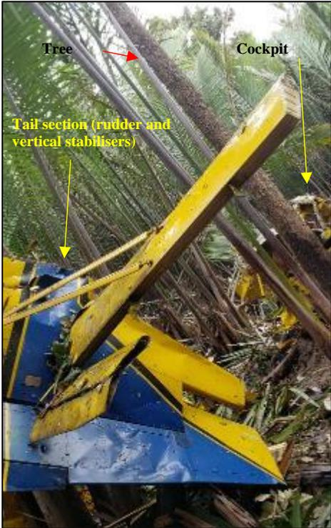
Figure 13: Tail section and cockpit with reference to the tree
