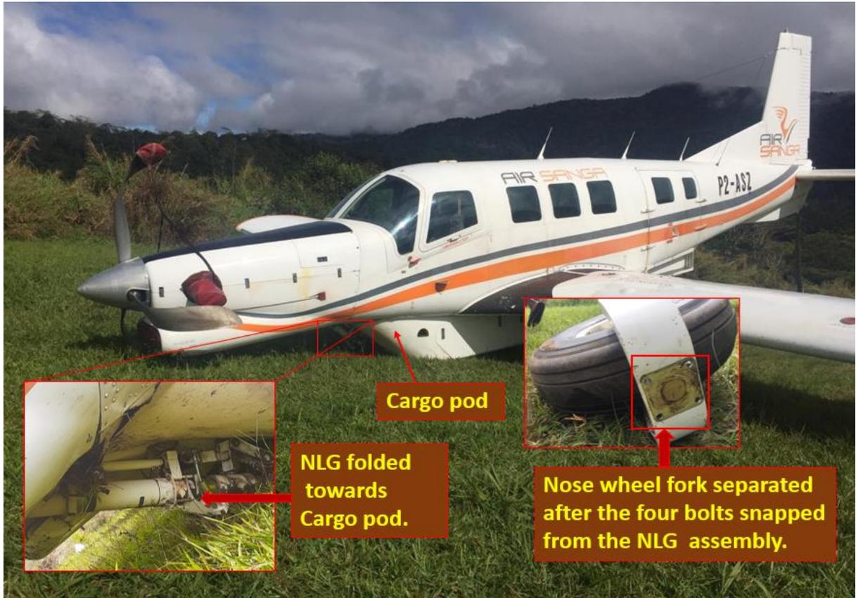
**Figure 3: The nose wheel separation and nose landing gear strut damage.**
