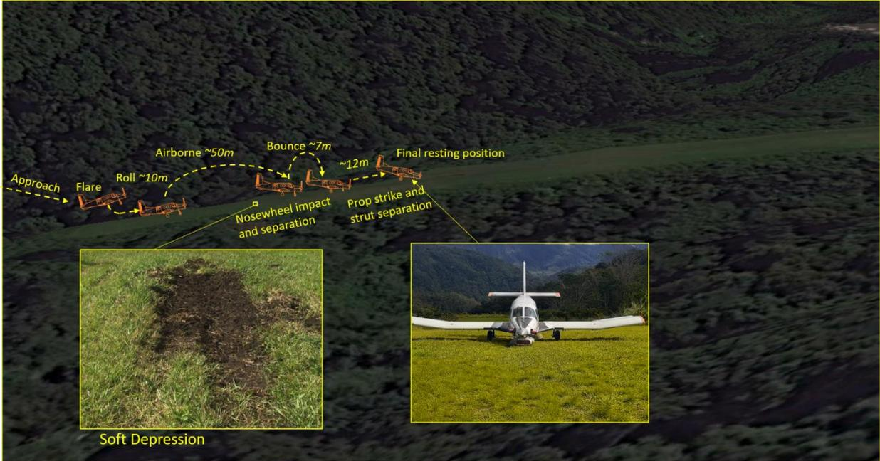
Figure 9: Aircraft touch down to the final resting position (not drawn to scale)
