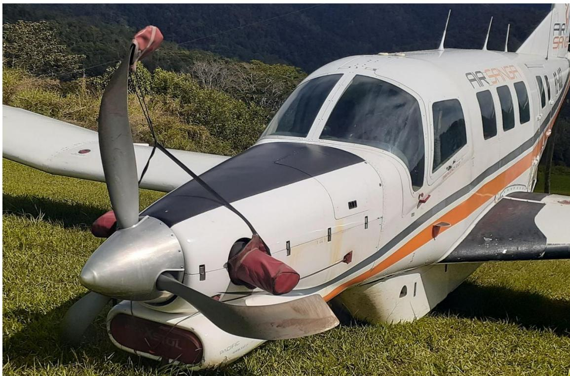
**Figure 4: Propeller damage.**
