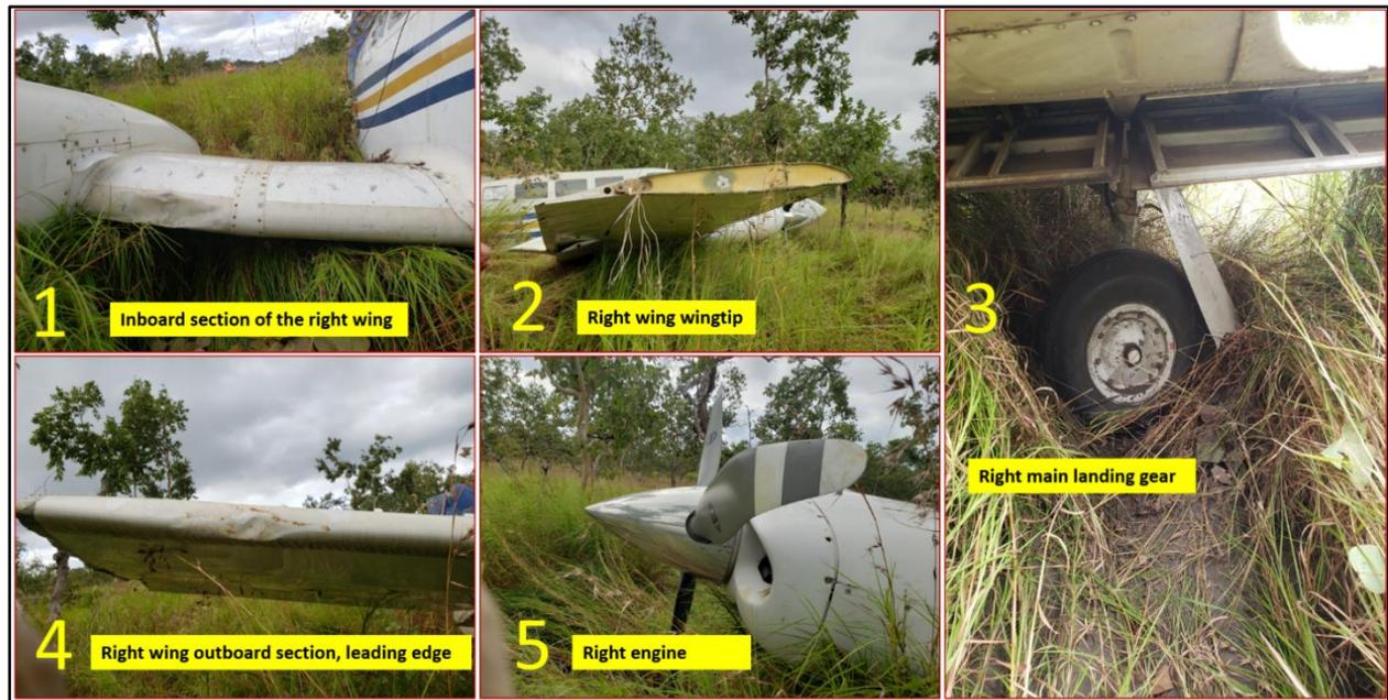
**Figure 5: Damage on the right wing**
