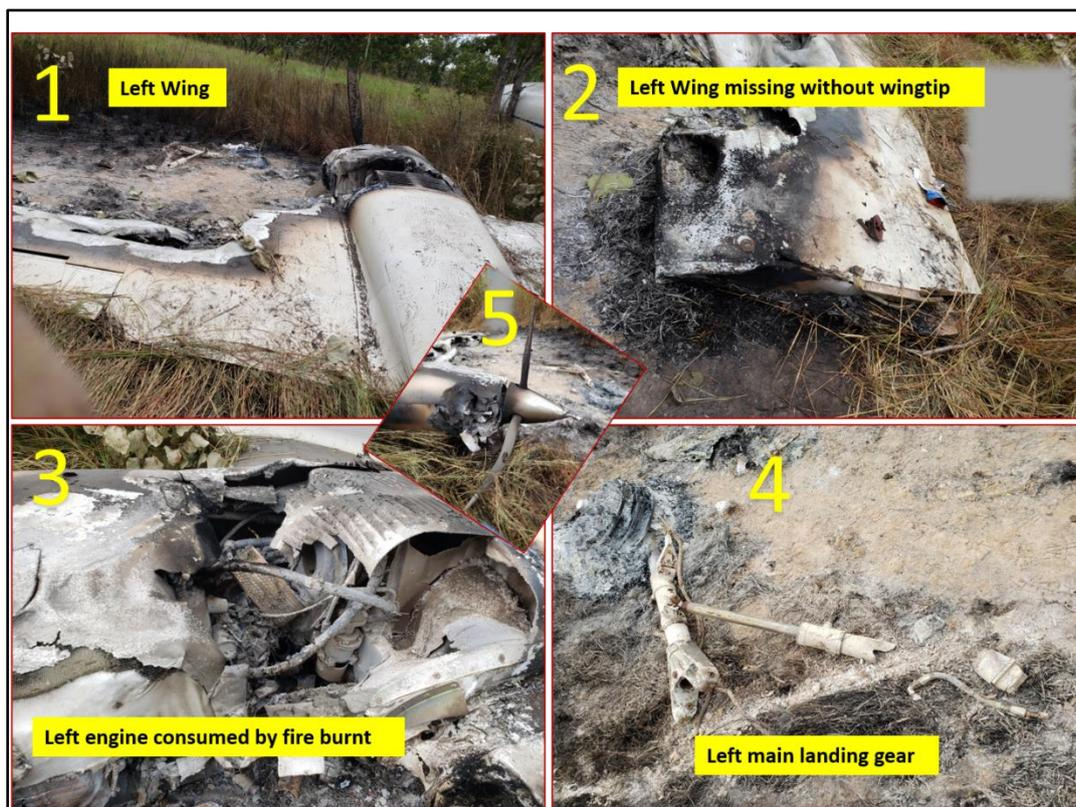
**Figure 4: Damage to left wing**
