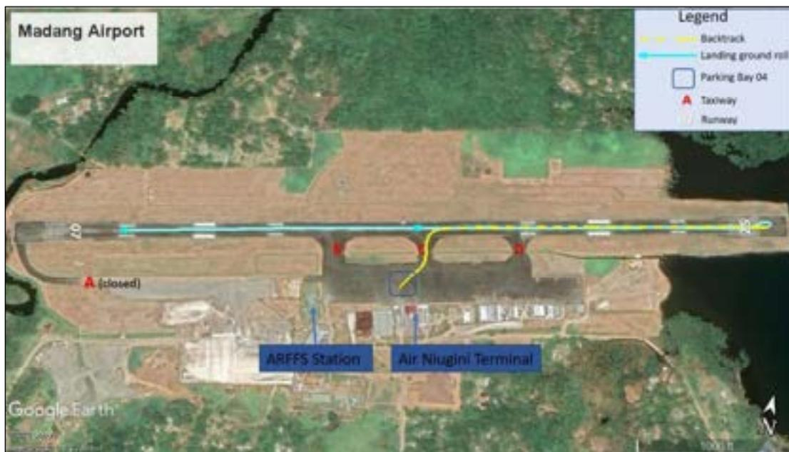
**Figure 9: Ground roll direction of the aircraft post touchdown at Madang Airport.**
