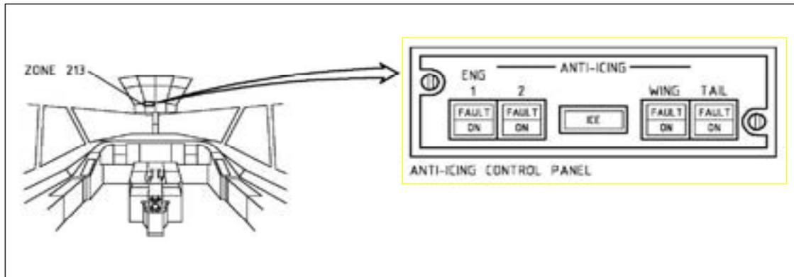
**Figure 4: Anti - icing panel**
