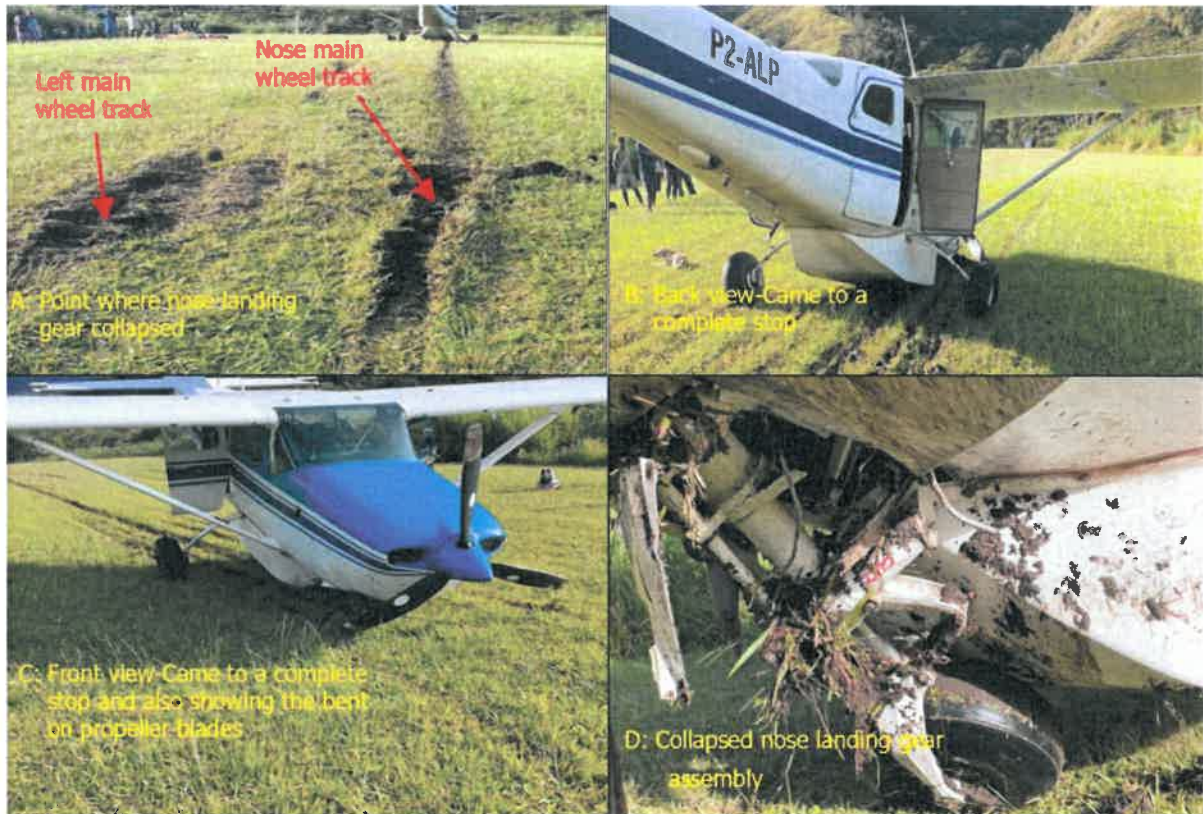
Figure 4: Impact and Damage overview
