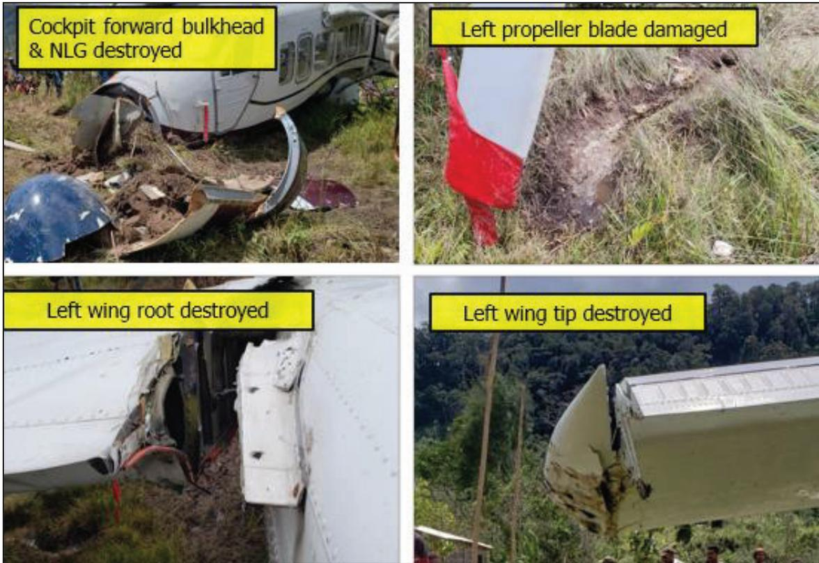
Figure 4 Damage sustained by P2-ASM
