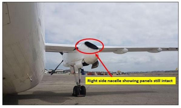
Figure 2: Right nacelle fully intact
