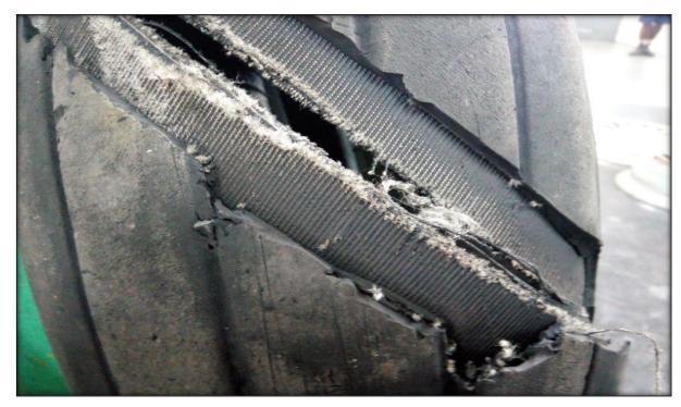
Figure 3: Damage number-2 left main wheel tyre
