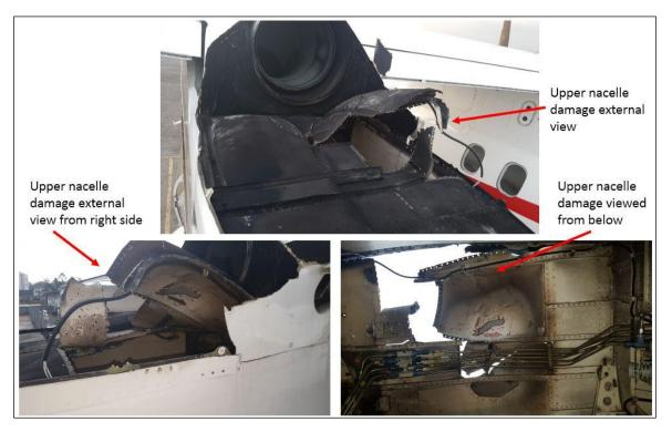
Figure 1: Damage area left nacelle
