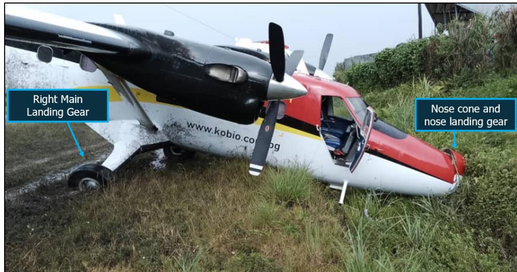
Figure 6: Damage to the nose area
