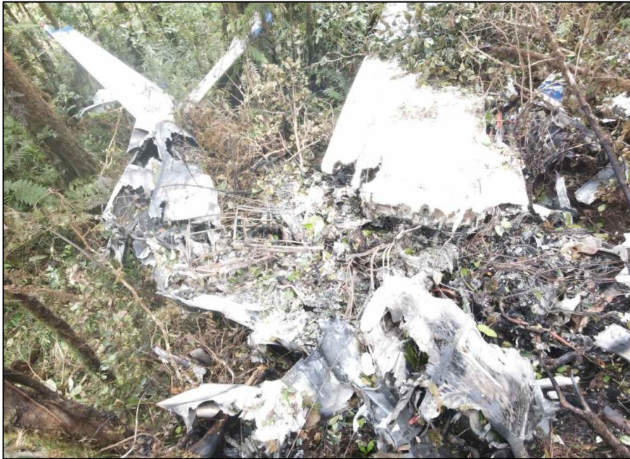
Figure 4: Aircraft destroyed by impact forces and fire. View looking back along final track
