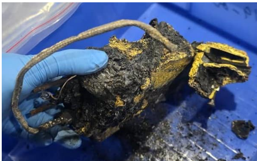
Figure 7: ELT destroyed by post-impact fire
