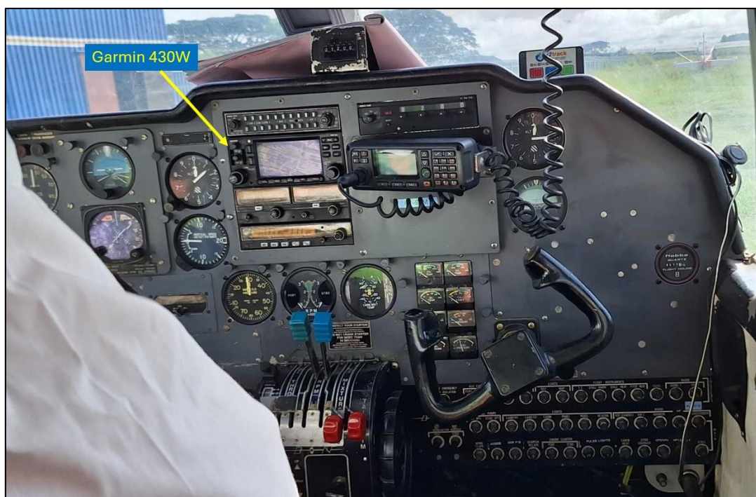
Figure 9: Instrument panel. Garmin 430W in centre console to right of flight instruments
