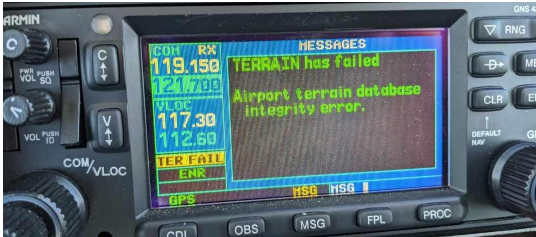
Figure 11: Garmin 430W receiver screen showing indicative terrain fail display
