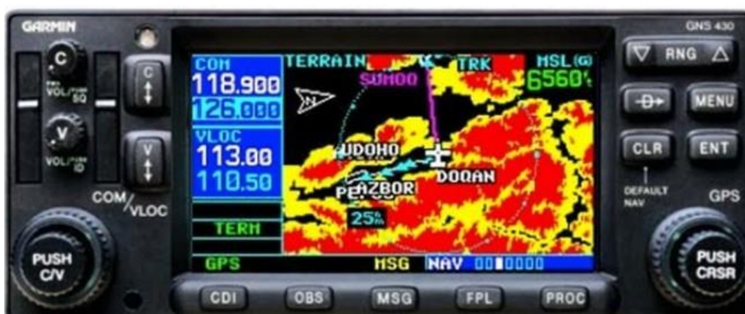
Figure 10: Garmin 430W receiver screen showing indicative terrain display
