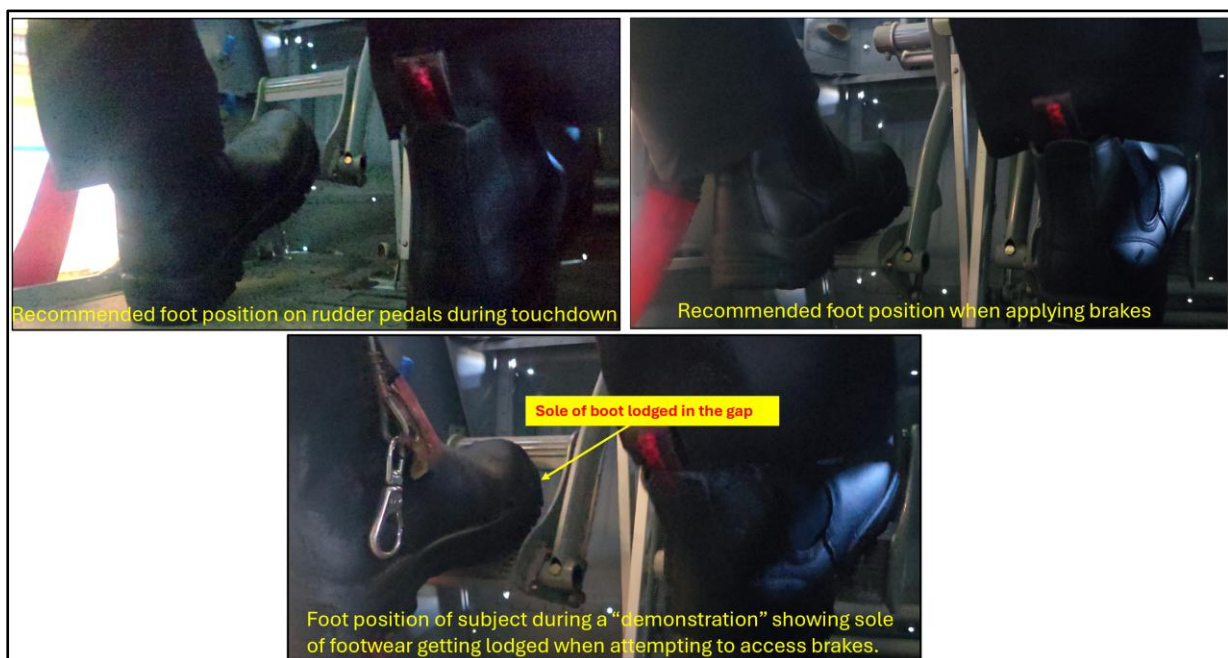
Figure 7: Demonstration of Foot/Feet position on Rudder Pedals and Brakes.
