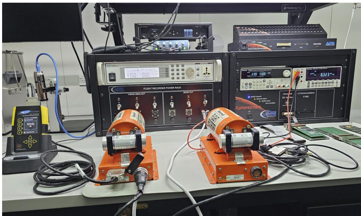
Figure 12: Download of the recorders at the AIC Flight Recorder Laboratory.
