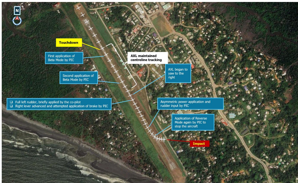
Figure 4: Illustration of P2-AXL tracking along the runway from touchdown to impact.
