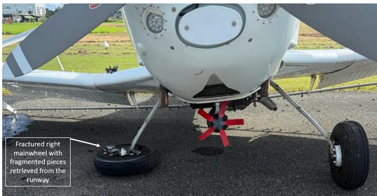
Figure 4: Damage sustained by VH-NAB
